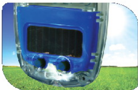
Integrated solar cell to extend battery life
