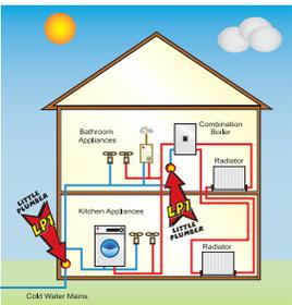
It doesn't matter where you install you LP unit as long as it is on the COLD mains pipe.
