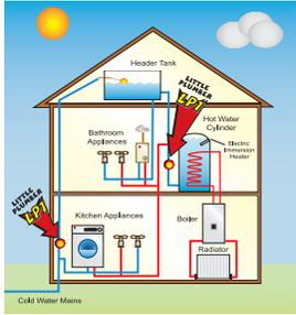
LP will only treat water if there is no break in the stream. With a cold tank in the loft, the water fills up through a ball valve so there is a break in the stream and the current injected by the LP cannot jump this gap. This means the water in the tank becomes untreated.
