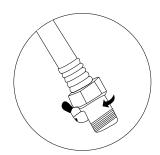
3. Attach the Nozzle with Shut-off Valve to one end of the Hose.
